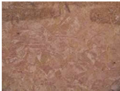
Figure 3. Micrograph of the heat affected zone of one of the welded areas.
