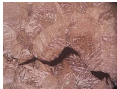
Figure 4. Micrograph of the hydrogen crack.
